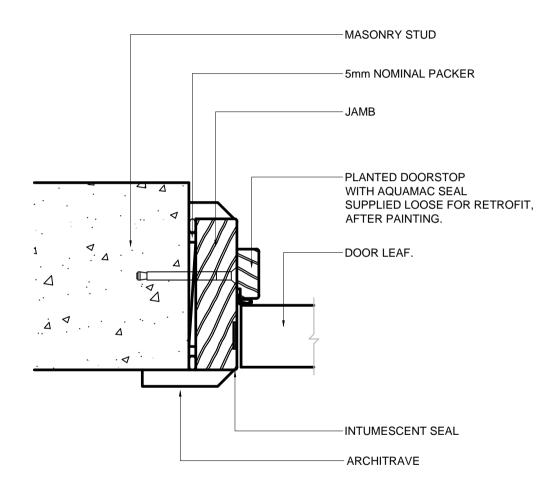
FILE NAME : Timber Jamb Install Masony Stud DETAIL : Installation for Timber Jamb into a Masonry Wall
