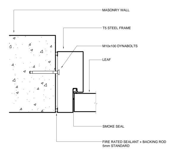
FILE NAME: T5 Steel Jamb Install Masony Stud DETAIL: Installation for T5 Steel Jamb into a Masonry Wall
