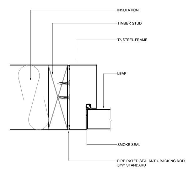
FILE NAME: T5 Steel Jamb Install Timber Stud DETAIL: Installation for T5 Steel Jamb into a Timber Wall
