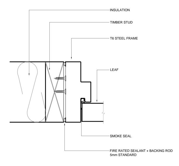
FILE NAME: T6 Steel Jamb Install Timber Stud DETAIL: Installation for T6 Steel Jamb into a Timber Wall
