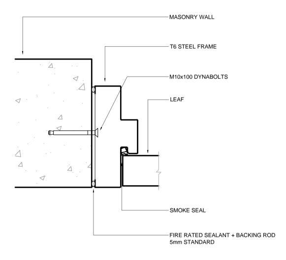
FILE NAME : T6 Steel Jamb Install Masony Stud DETAIL : Installation for T6 Steel Jamb into a Masonry Wall
