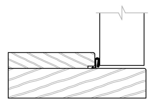
FILE NAME: T1 Jamb DETAIL: Flat Timber Jamb with FULL WIDTH Stop and GAQ seal
